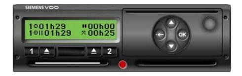
On the image above we will use the large circular button that has the 'up arrow head', 'down arrow head', 'left arrow - with a dot at its point' and the right hand button marked 'OK'.
